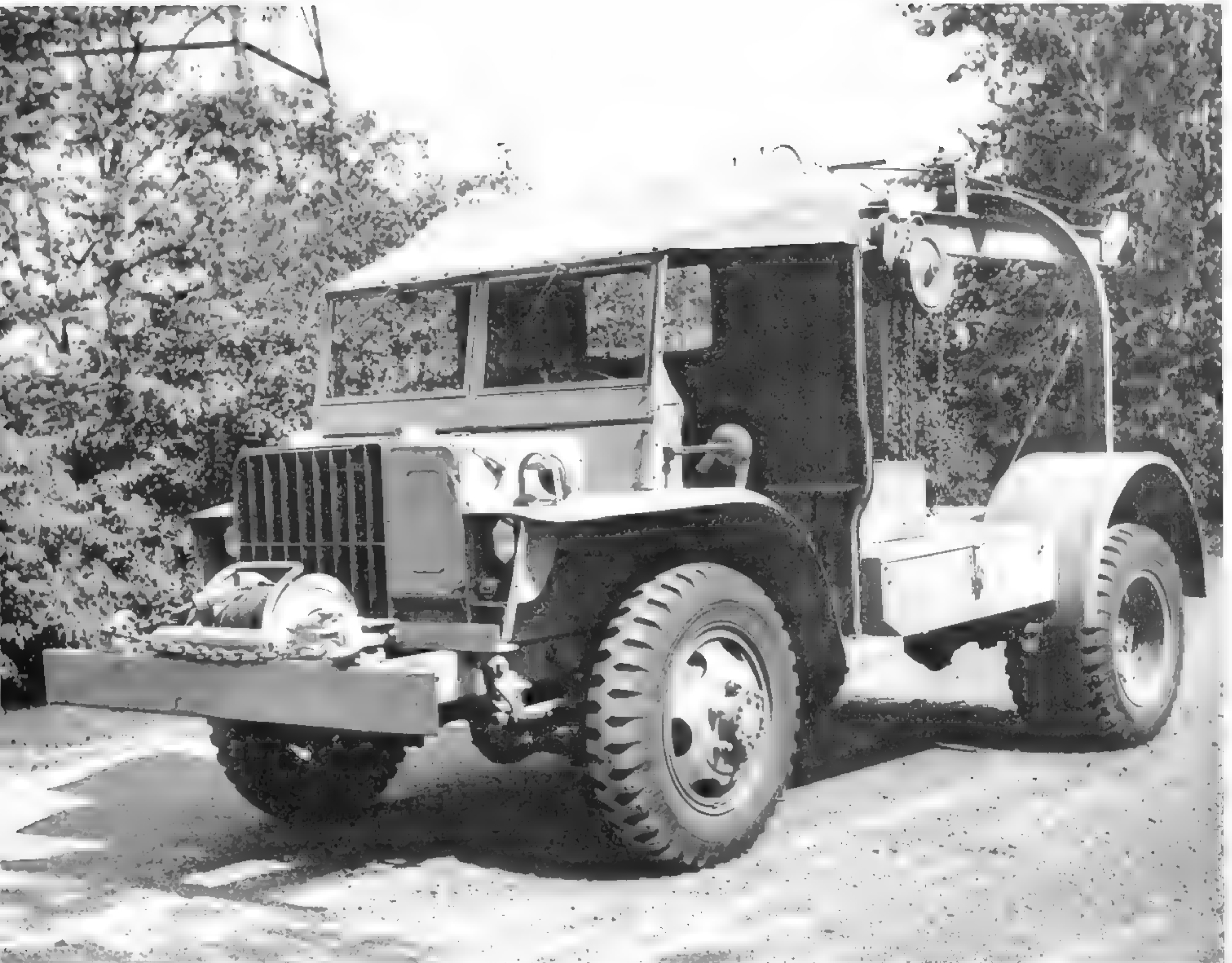
The improved Bomb Service Truck, the GTBC, reverted to the dual rear wheels used by the rest of the series, and included a front winch. This winch was the Braden MU-5A model, but the Gar Wood unit was also fitted, and was preferred. This model accounted for about 50 percent of the Navy's GTB series purchases. (Photo courtesy of the Bryce Sunderlin collection)
